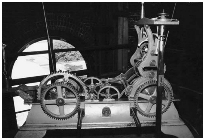
Figure 1, left. The Cabell County Courthouse in Huntington, WV. Figure 2, below. E. Howard time and strike movement, inside the Cabell County Courthouse tower.
