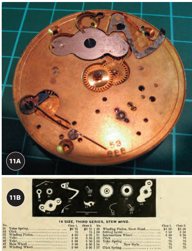
Figure 11. (A) The second-generation setting mechanism and the first lever-set rocking yoke style setting mechanism. PHOTO BY GEORGE MEYER. (B) The associated parts list from Green Bros., Maiden Lane, NY, Illustrated Price List, 1889.
