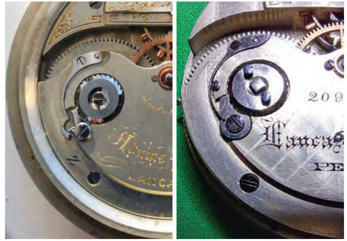
Figure 3. The first model click spring assembly (left) and second model (right). Moseley's click design was a better design: it was easier and simpler to manufacture plus it included a let-down screw. PHOTOS BY GEORGE MEYER.
