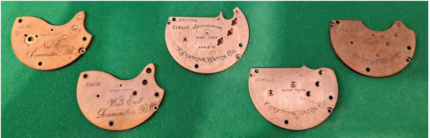
Figure 13. These are top plates used over the life of the ébauche. From left to right, early key wind, a stem-wind/lever-set, dustproof 15-jewel, a top plate made from a dustproof plate without the dustproof feature, and a flat-top shape. PHOTO BY GEORGE MEYER.
