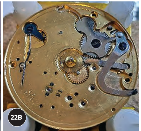
Figure 22. An example of a 24-hour dial (A) and the hour gearing required (B), which converted the watch to time correctly. PHOTOS BY GEORGE MEYER.
