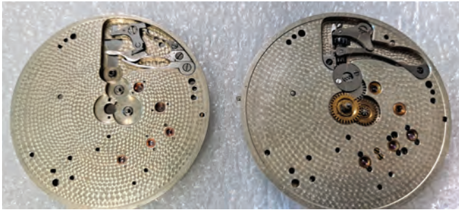
Figure 2. Note the difference in first model (left) and second model (right) setting mechanisms. Moseley's design, in the second model, uses fewer parts, requires less material and machining, and in our opinion is more robust. It is clearly superior to the Perry design. PHOTO BY GEORGE MEYER.
