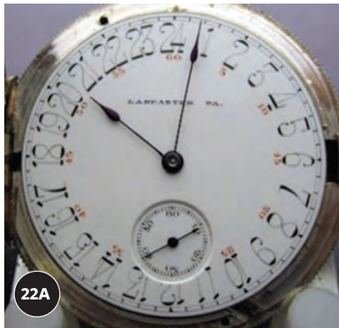
Figure 22. An example of a 24-hour dial (A) and the hour gearing required (B), which converted the watch to time correctly. PHOTOS BY GEORGE MEYER.
