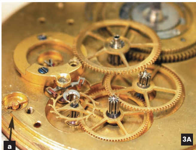
Figure 3. Arrangement of train wheels of E. H. & Co. Model 1862N movement: A. Thick plate movement, with (a) showing the countersinking of the dial pin, necessitated by the thicker plate; B. Thin plate movement. PHOTOS BY JOHN WILSON.
