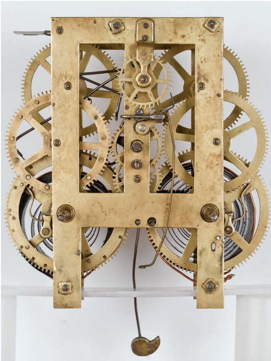
Figure 12A. Front of a "Square Nut" striking movement with a 6-spoke escape wheel. AUTHOR'S PHOTO.
