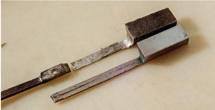
Figure 7. Original detent foot (top) and new detent foot (bottom). PHOTO BY DAVE COOPER.
