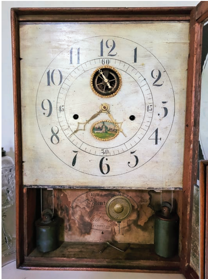
Figure 18. Restored clock with a remade dial and hands, with the door open. AUTHOR'S PHOTO.
