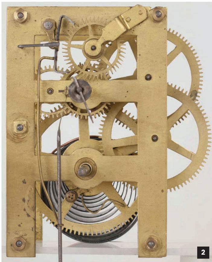
Figure 1B. (top left) Front left plate leg belonging to the "Square Nut" movement in Figure 1A. AUTHOR'S PHOTO. Figure 1C. (top right) Anglo-American-styled drop-dial case containing a "Square Nut" striking movement with a 5-spoke escape wheel in Figure 1A. AUTHOR'S PHOTO. Figure 2. (bottom) Front of a "Square Nut" timepiece movement with a 5-spoke escape wheel. AUTHOR'S PHOTO.
