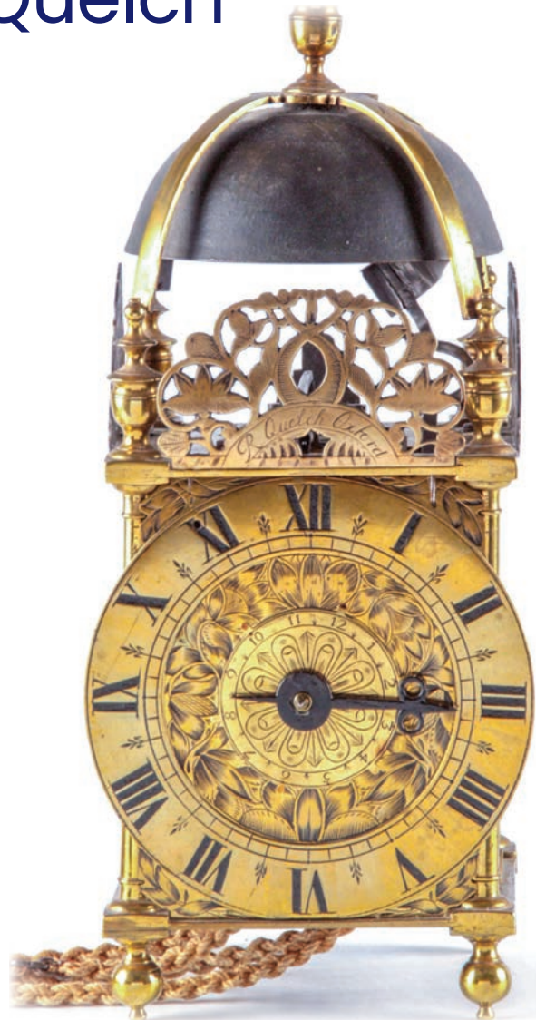
Figure 1. Front view of the Quelch clock, pre-restoration. The dial shows the typical second-period shading of the tulip flowers and the half hour markers. Note the canon pinion and minute-hand shaft for the hands and the unsuitable replacement hand. PHOTO BY GEOFF COX.
