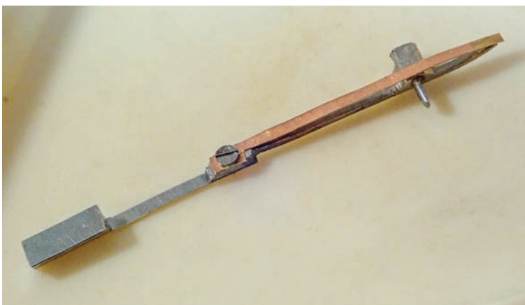
Figure 9. Completed detent assembly. PHOTO BY DAVE COOPER.
