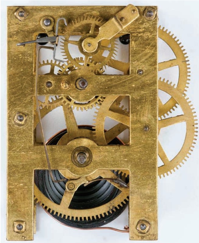
Figure 8A. Front of a "Square Nut" timepiece movement with a 4-spoke escape wheel and "Small Square Nuts." AUTHOR'S PHOTO.
