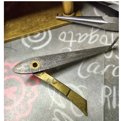
Figure 1. The lifting lever needed some cleanup from previous soldering. PHOTO BY PAUL KRAUS.
