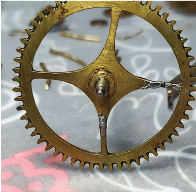
Figure 2. The gathering wheel was broken in two of its four spokes. The wheel was thoroughly cleaned and resoldered—with much less solder! PHOTO BY PAUL KRAUS.
