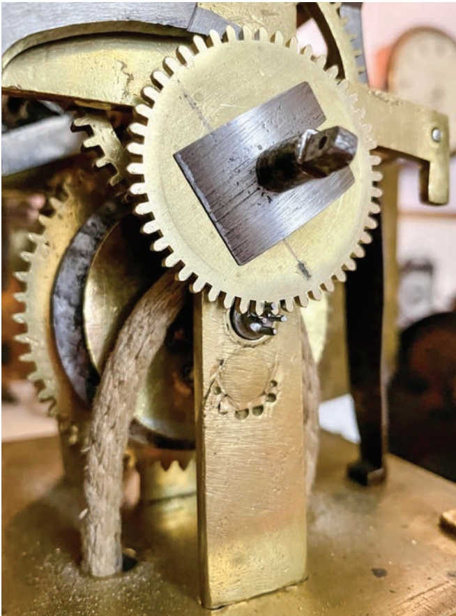
Figure 12. Replacement pinion of report/cut-down hour and star wheel assembly. PHOTO BY GEOFF COX.
