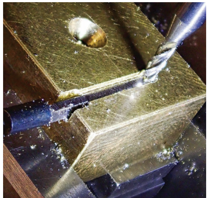
Figure 10. Purpose-made machining fixture. PHOTO BY DAVE COOPER.
