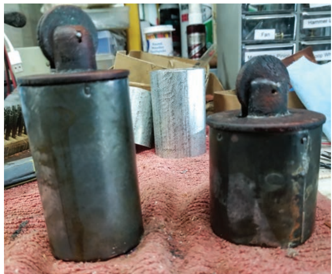
Figure 13. Picture of two proper, different sized weights made using methods from the Cog Counter's Journal . AUTHOR'S PHOTO.
