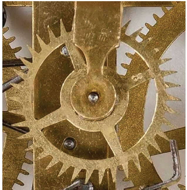
Figure 3D. Escape wheel of the "Square Nut" movement in Figure 3A with "8" punched on the spoke at the 2 o'clock position. AUTHOR'S PHOTO.
