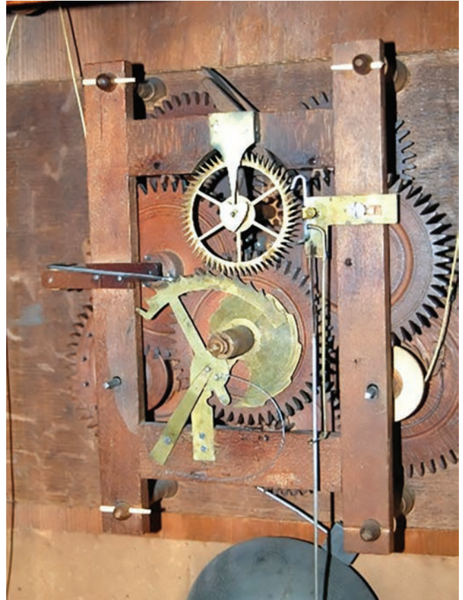
Figure 2. Model 1-C rack-and-snail-strike movement. AUTHOR'S PHOTO.
