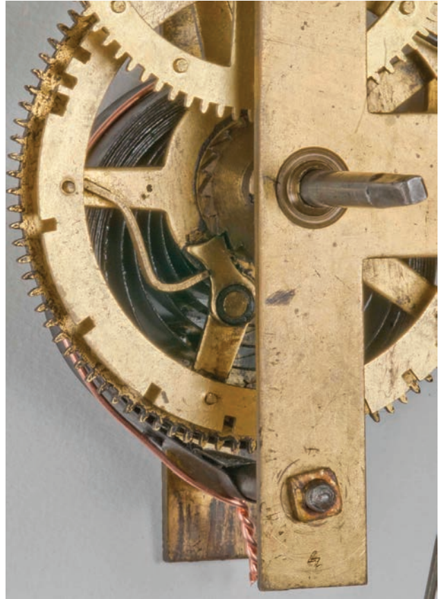
Figure 3C. Front left plate leg of the "Square Nut" movement in Figure 3A. AUTHOR'S PHOTO.
