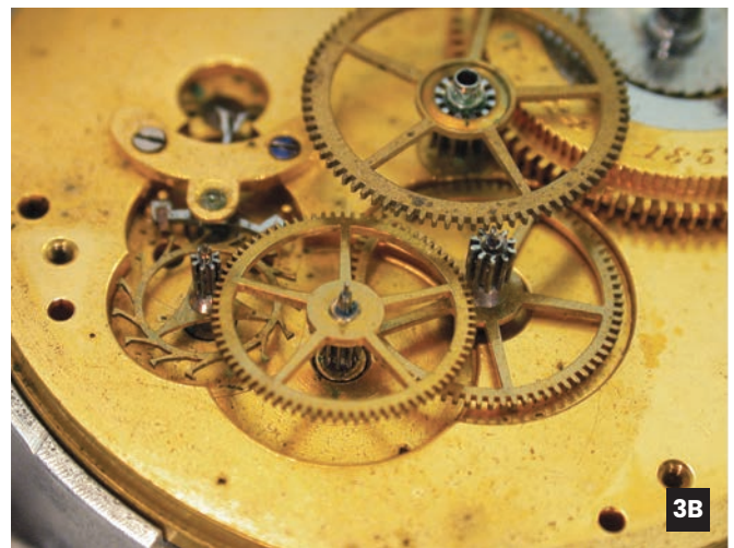
Figure 3. Arrangement of train wheels of E. H. & Co. Model 1862N movement: A. Thick plate movement, with (a) showing the countersinking of the dial pin, necessitated by the thicker plate; B. Thin plate movement. PHOTOS BY JOHN WILSON.
