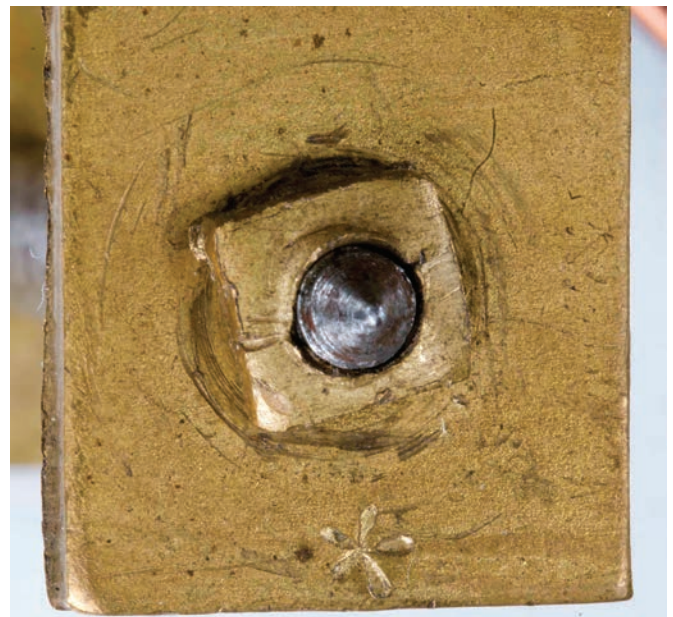
Figure 9. A punched leg mark that looks like five petals from a "Square Nut" timepiece movement with a 4-spoke escape wheel. Note the "Small Square Nut." AUTHOR'S PHOTO.
