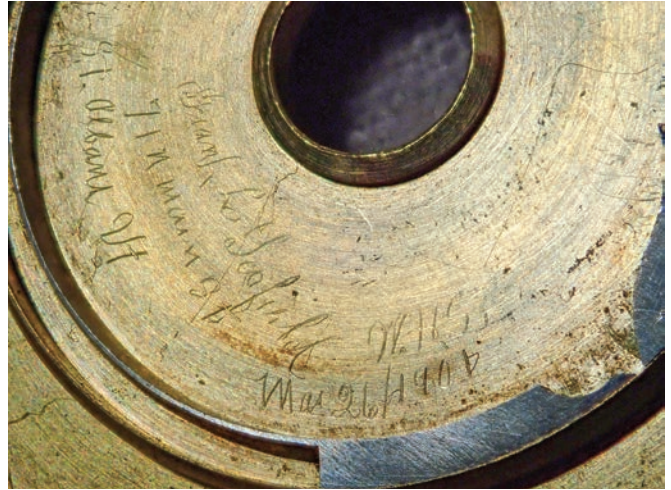
Figure 13. Hand-scratched markings on the movement under the dial. PHOTO BY DAVE COOPER.
