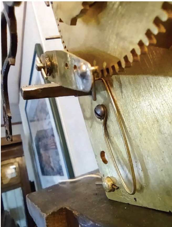
Figure 3. The rack tailpin was previously soldered but still loose in the rack tail. It was resoldered and much solder was removed. PHOTO BY PAUL KRAUS.
