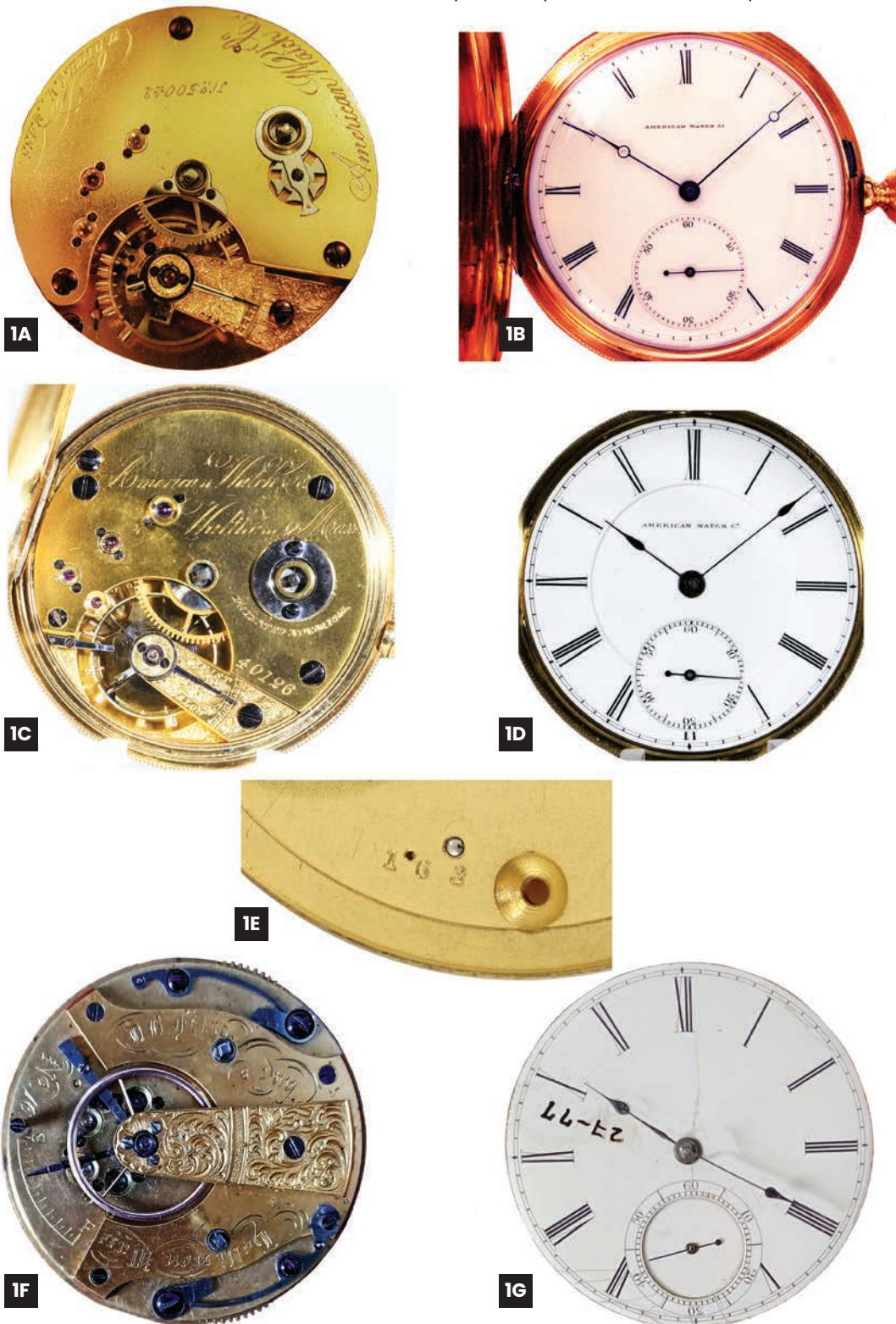
Figure 1. A. A.W. Co. grade 18-size Waltham Model 1859 movement No. 40,126, with D. B. Fitts’s patented reversing center pinion (concentric with the center wheel pinion); B. Dial of No. 40,126; C. A.W. Co. grade Model KW20 movement No. 50,042 with N. P. Stratton’s safety barrel. D. Dial of movement No. 50,042; E. N.W. Co. assembly number, 163, on the underside of the dial plate of the ébauche that ultimately was finished as A.W. Co. movement No. 50,042. PHOTOS IN 1A-1E BY CLINT GELLER; F. Movement No. 16 of 17 22-size 8-day movements with tandem mainsprings produced by the partnership of Edward Howard, David P. Davis, and Aaron L. Dennison at the American Horologe Co. (A.H. Co.). Movement Nos. 16 and 17 are signed “D. B. Fitts, Holliston Mass.”, and have cylinder escapements, indicating that Fitts likely received these two movements in an incomplete state and finished them after they left the Roxbury factory; G. Dial of No. 16 finished ca. 1851 by A.H. Co. PHOTOS IN 1F-1G COURTESY OF THE NATIONAL WATCH & CLOCK MUSEUM.
