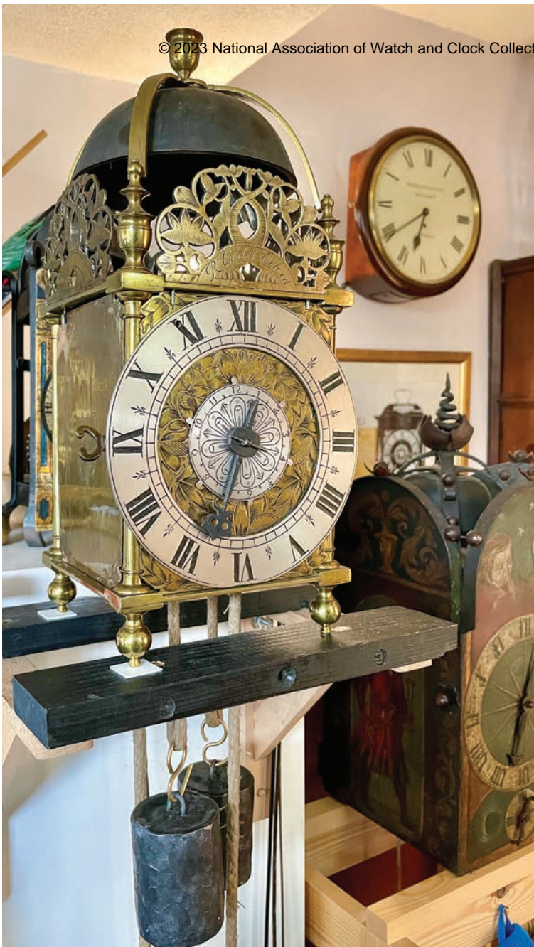
Figure 14. The finished Quelch clock awaiting the second phase: the crown-wheel balance reinstatement. PHOTO BY GEOFF COX.
