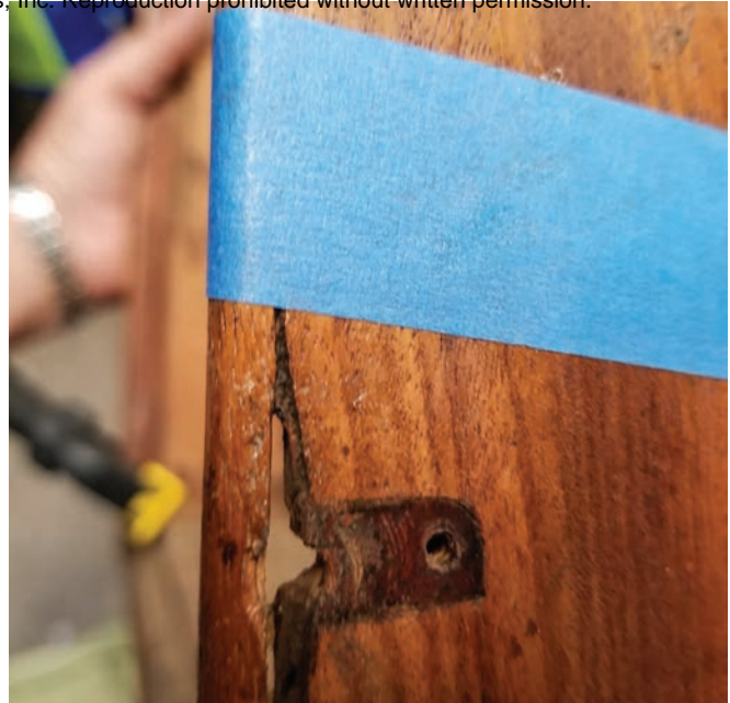
Figure 12. Sadly, all that remains of the original finish was this strip, about 10mm x 25mm, found under the repair attempted on the lower hinges. AUTHOR'S PHOTO.
