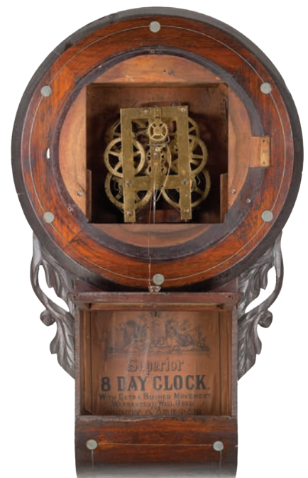
Figure 3G. Another view of the case in Figure 3E with the dial and bezel removed to show the dial surround permanently fixed with screws, and the full-width trunk door tied open to show the label. AUTHOR’S PHOTO.
