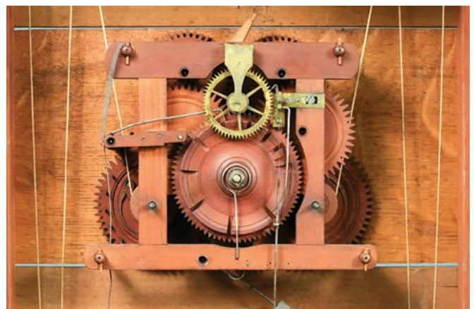
Figure 3. Model 2 count-wheel strike. This was the immediate successor to the rack-and-snail version in my 1-C example. AUTHOR'S PHOTO.
