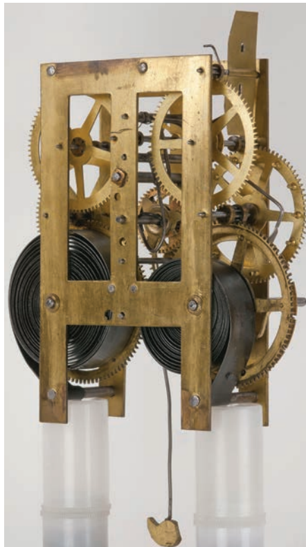
Figure 3A. Front of a "Square Nut" striking movement with a 4-spoke escape wheel. AUTHOR'S PHOTO.
