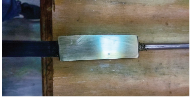
Figure 6. The suspension block with brass shims soldered into place. PHOTO BY PAUL KRAUS.
