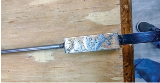
Figure 5. Soldering additional brass onto the suspension block. PHOTO BY PAUL KRAUS.
