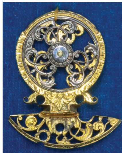
Figure 11. Early 18th-century watch cock with silver inlay in the table. From the Bates collection at the AHS headquarters in London. PHOTO BY DR. JAMES NYE, USED BY PERMISSION OF THE ANTIQUARIAN HOROLOGICAL SOCIETY.
