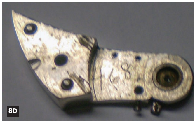
Figure 8A. An open-face 16-size, 17-jewel movement; B. A hunting 16-size, 17-jewel movement. PHOTOS IN 8A–B COURTESY OF ARNIE VANTIEM. C. A bridge with a movement serial number; D. No. “468” scratched on the bottom of the balance cock. AUTHOR’S PHOTOS.
