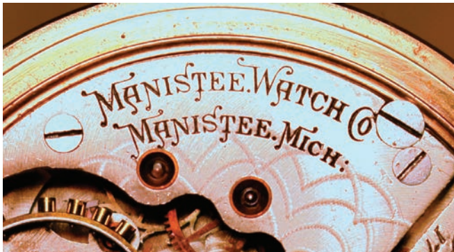
Figure 10. Close-up photo illustrating the cap jewel on the escape wheel. COURTESY OF LONNIE ROBERTS.
