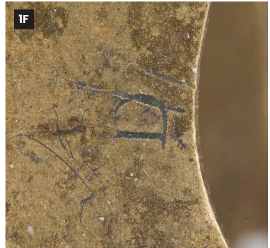
Figure 1F. Enlargement of the punched "D" mark seen in Figure 1E from the movement in Figure 1A. AUTHOR'S PHOTO.
