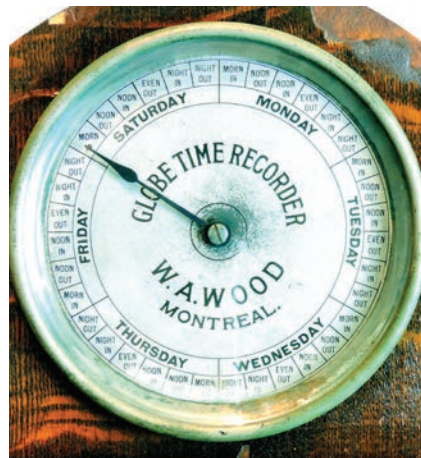
Figure 7. The upper dial that shows the days of the week: Monday to Saturday, but not Sunday.
