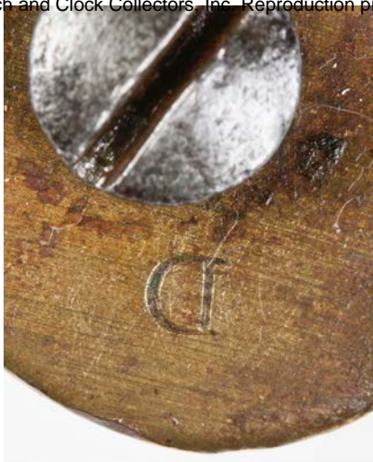
Figure 2. Enlargement of a punched "D" mark found on a "The Caledonian Registered Vienna" movement. AUTHOR'S PHOTO.
