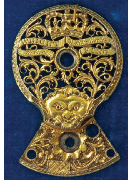
Figure 6. Late 18th-century watch cock with a watchmaker's name: "Wright Watch Maker to the King". From the Bates collection at the AHS headquarters in London. PHOTO BY DR. JAMES NYE, USED BY PERMISSION OF THE ANTIQUARIAN HOROLOGICAL SOCIETY.
