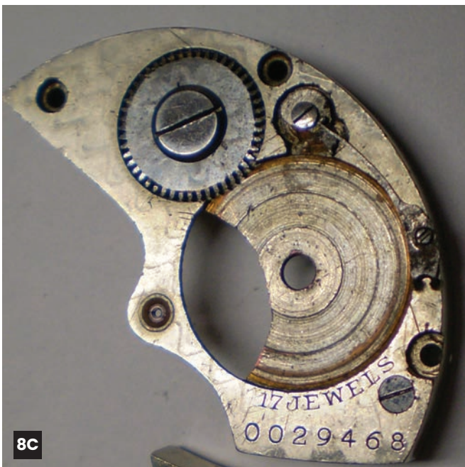
Figure 8A. An open-face 16-size, 17-jewel movement; B. A hunting 16-size, 17-jewel movement. PHOTOS IN 8A–B COURTESY OF ARNIE VANTIEM. C. A bridge with a movement serial number; D. No. “468” scratched on the bottom of the balance cock. AUTHOR’S PHOTOS.
