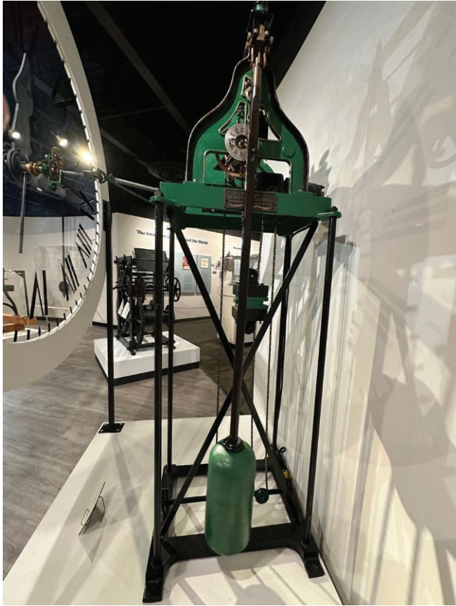
Figure 14. A Seth Thomas no. 6 mechanical clock with electric winding at the National Watch & Clock Museum. This is the same type of clock that Hamilton purchased in 1910 for the new East Tower wing and factory entrance. It is a perfect fit for the wood box still in the tower. PHOTO BY MICHAEL SCHWARTZ.
