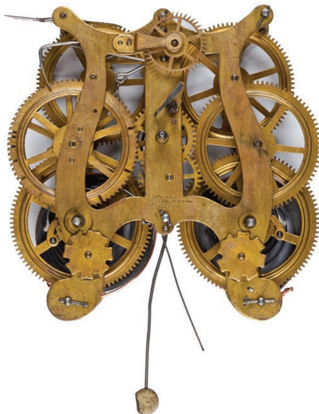
Figure 1. Front of the movement with lyre-shaped plates, name-punched "S. Thomas / Plymouth Conn / USA". AUTHOR'S PHOTO.
