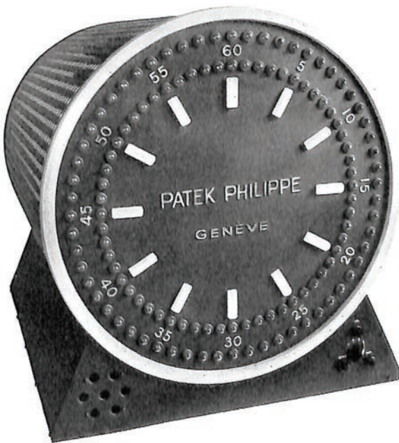
Figure 5. Patek Philippe quartz clock from 1952 in Journal Suisse d'Horlogerie . This clock has no wheels and no hands: markers light up on the dial to tell the time.
