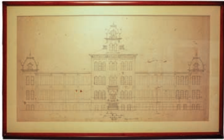
▲ Figure 2A. This is the original line drawing of the factory by architect Clarence Luther Styles in 1874. It is marked "Drawn at Zahm's Corner" and depicts what was intended to be built. Shortfalls in initial capital prevented a clock and end cupolas from being completed. This artifact provided many answers to our early questions. COURTESY OF THE NATIONAL WATCH & CLOCK MUSEUM. PHOTO BY MICHAEL SCHWARTZ.
