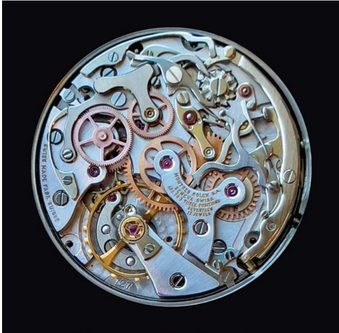
Figure 5. Owen's favorite chronograph movement: the Valjoux cal 72 upgraded by Rolex to cal 727 for an early Rolex Cosmograph Daytona. AUTHOR'S PHOTO.
