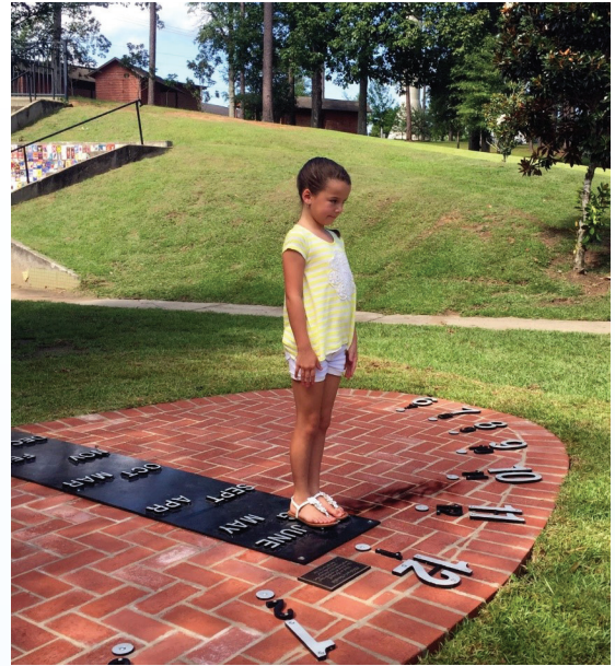
An analematic sundial, where a person becomes the gnomon and their shadow tells the time. © North American Sundial Society.
