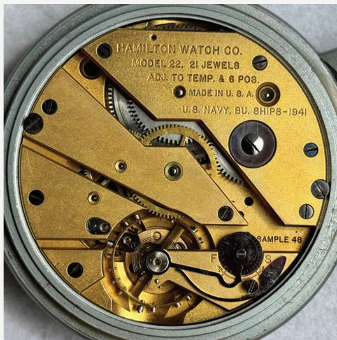
Figure 7. The dial, case, movement, and wheel of the Hamilton M22 prototype marked "Sample 48" and dated 1941. PHOTOS COURTESY OF RHETT LUCKE.
