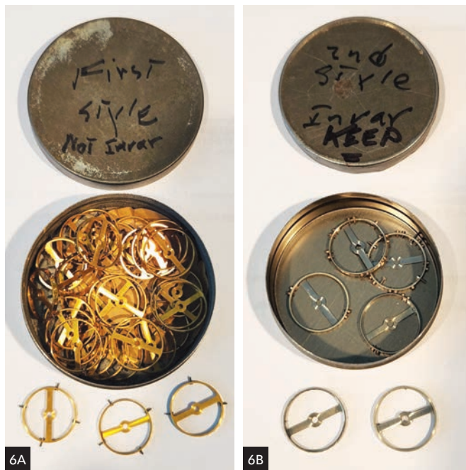
Figure 6. These two "new old stock" tins of M22 balance wheels show that there was enough of a difference to warrant separation. A. The "First Style" tin clearly states "Not Invar", meaning these are the early gold-color balance wheels. B. The "2nd Style" tin states "Invar KEEP", meaning when these were presumably sent out to M22 repairmen, they were to use these new nickel steel/invar balance wheels when repairing M22s. PHOTOS COURTESY OF PAUL KRITCHEN.
