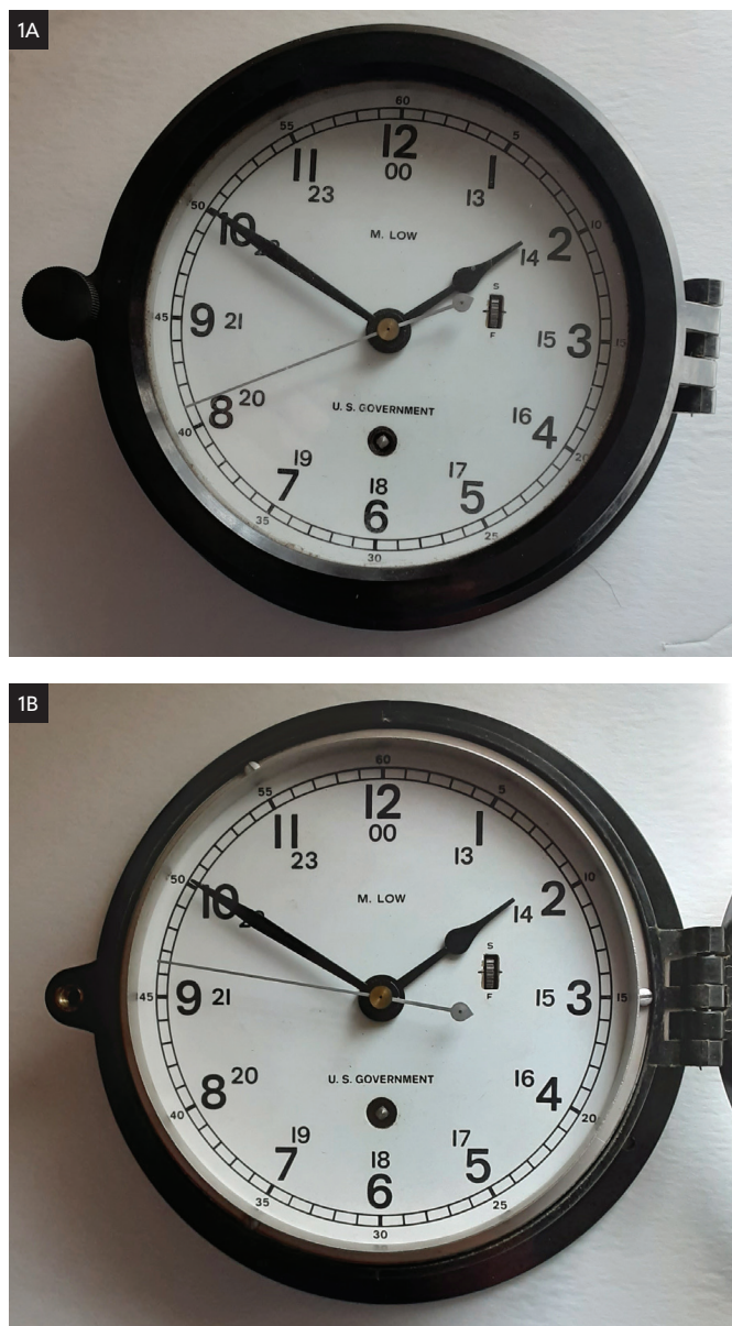
Figure 1. A 6" bulkhead clock with a white dial signed "M. Low U.S. Government", showing the bezel closed and opened. AUTHOR'S PHOTOS.
