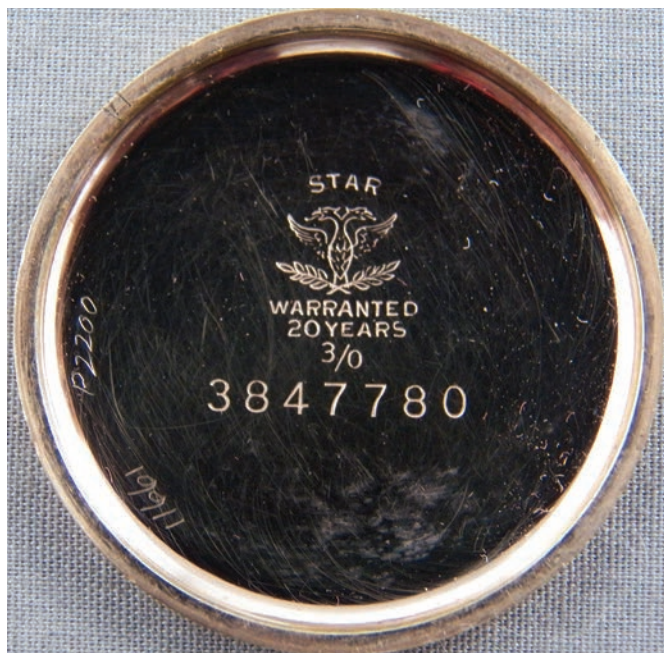
Figure 5. The inside of the case is marked "STAR" and states a size of 3/0 and a warranty of 20 years (gold-filled quality). The case back and bezel are the screw-on variety, which is somewhat unusual for a small case from this era, but would be more dust resistant than a more typical hinged case back and snap-on bezel. AUTHOR'S PHOTO.
