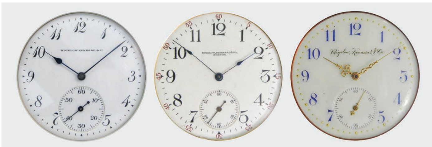
Figure 16. Other 12-size dials: The dial on the left is an early (1904) dial from the O'Hara Dial Co. The middle dial is a very common Waltham pattern but uncommon for BK&Co. On the right is a fancy dial with blue numbers and gold minute markers; the seconds dial is pressed rather than a separate piece. AUTHOR'S PHOTOS.
