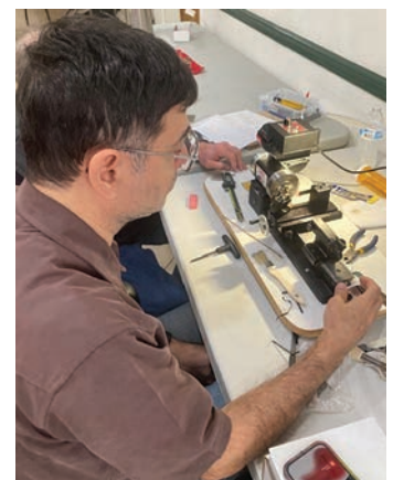
Figure 2. Daniel Demcovici using his Sherline lathe x-axis control knob to turn a KWM L19 bushing. AUTHOR'S PHOTO.
