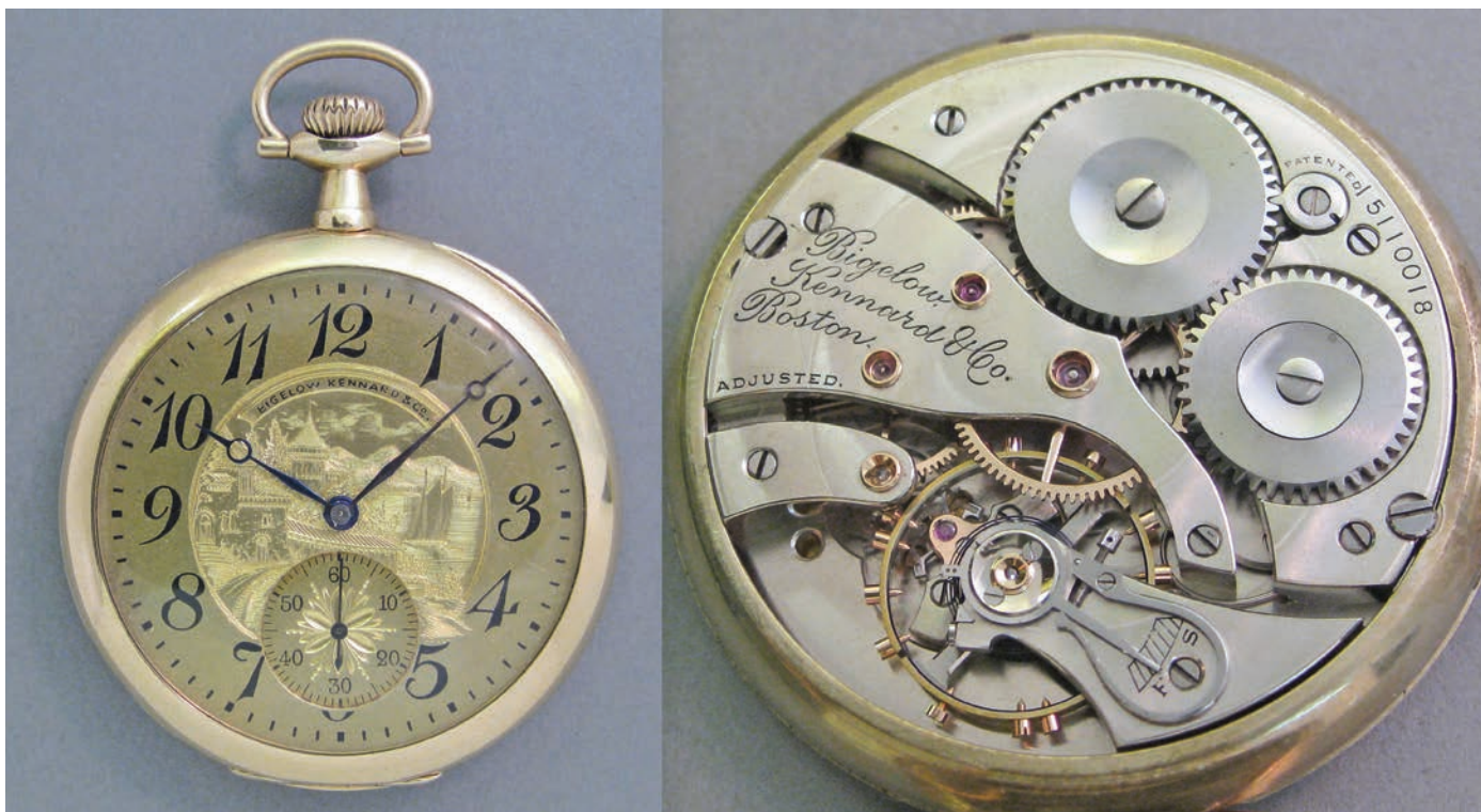
Figure 13. An example of a Colonial Series watch for BK&Co using a gilt metal scenic dial attached per Ohlson's 1907 patent (see Figures 17 and 18). This is a 23-jewel Riverside Maximus grade movement, No. 15,110,018; the case is not original. AUTHOR'S PHOTOS.
