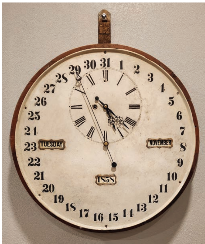
Figure 5. A dial with separate arbors used by the Calendar Clock Company gallery clocks. AUTHOR'S PHOTO.
