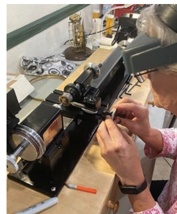
Figure 4. Beth Collier tipping the teeth on her project escape wheel, once the teeth were straightened and trued. AUTHOR'S PHOTO.
