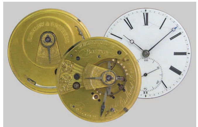
Figure 3. An example of an early English key-wind movement imported by Bigelow & Brothers (ca. 1840–46). This movement has a fusee and right-angle lever escapement. These were likely imported as uncased movements (to avoid extra tariffs for complete watches) and then cased domestically. AUTHOR'S PHOTO.
