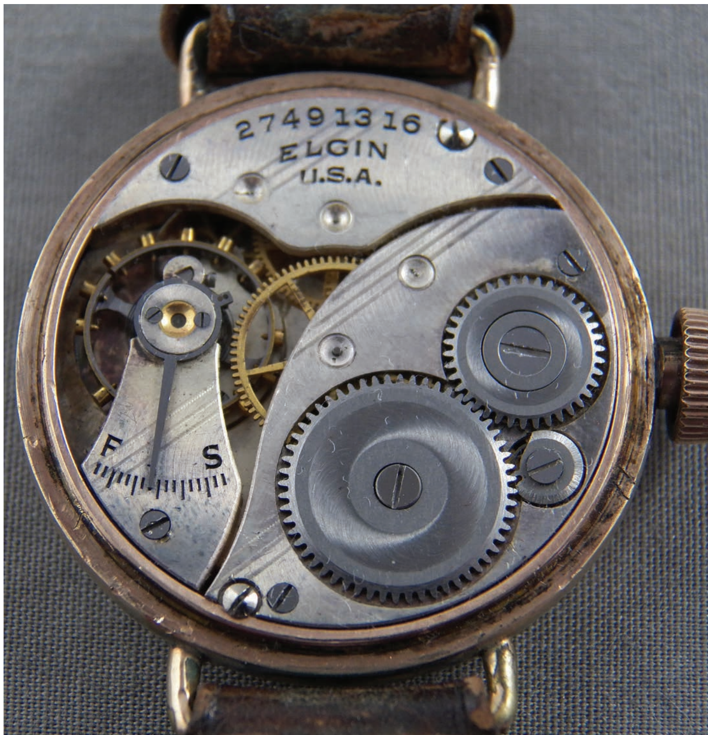
Figure 3. The movement for the Denver Parco Air Race watch is a fairly pedestrian quality grade 462 with 7 jewels and was made ca. 1924. Note the heavy, solid lugs and possibly original oversized crown. AUTHOR'S PHOTO.
