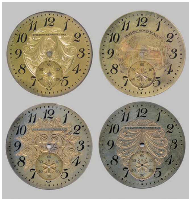
Figure 19. These are four pieces of a larger lot of custom, footless gilt metal dials that were never installed. Each dial was individually hand-engraved. See also Figure 20. AUTHOR'S PHOTOS.
