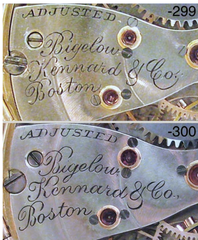
Figure 10. A comparison of two consecutive movements (11,032,299 and 11,032,300) shows differences in the engraved signature, which indicate these were hand engraved. Note, for instance, the letter "g" and the "Co." The signatures on later movements were more consistent and likely stamped with dies. AUTHOR'S PHOTOS.
