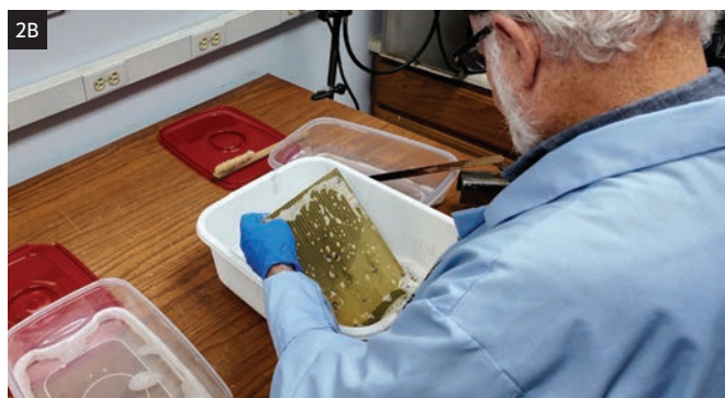
Figure 2A. Plate disassembly: Rory loosening one of the large blue screws holding the formidable front and back plates together, with Ken holding and stabilizing the assembly. B. Cleaning of the clock movement: Ken hard at work cleaning one of the plates and ensuring that all pivot holes are completely free of the solidified lubricant last used in the clock. There was no liquid lubricant left in the clock movement; it had turned into a sticky, waxy, green goo. PHOTOS BY ALEX SIMPKINS.
