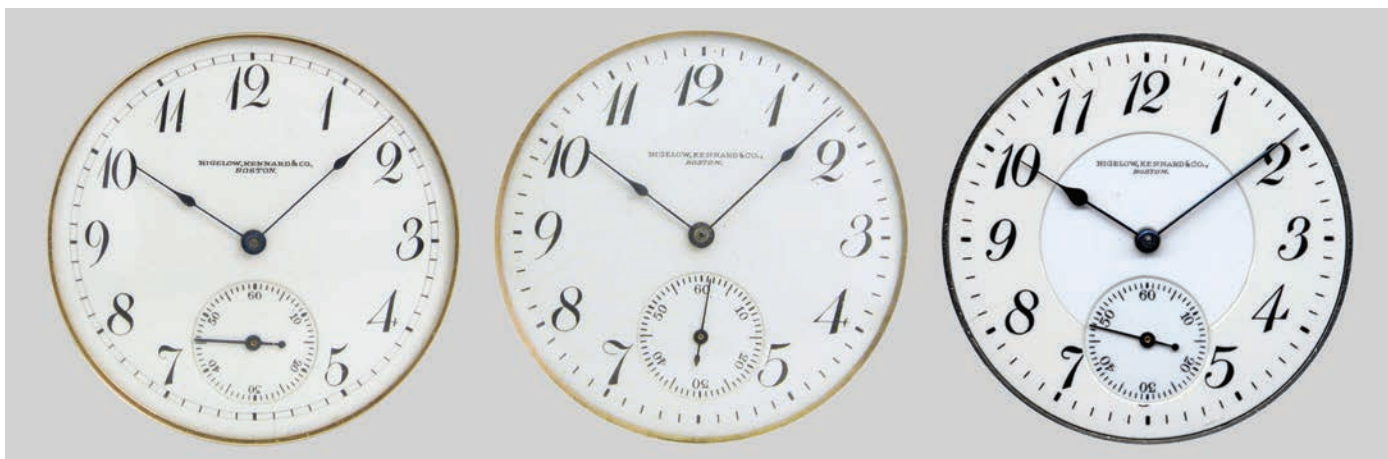
Figure 14. The majority of movements for BK&Co used the Empire pattern dial (left and center) with some variation in weight and slant as well as ring track or (later) hash marks for the minutes. Hull pattern numerals (right) were used on many later movements. Shown here is a double-sunk version used on some 23-jewel watches. AUTHOR'S PHOTOS.
