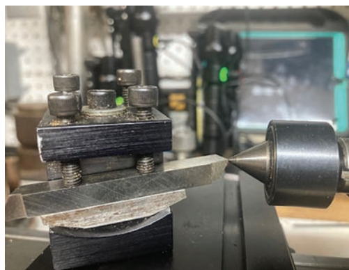
Figure 3. Shown here is the method to ensure that the Sherline lathe graver bit is perfectly aligned to the center of cutting stock. For facing round stock, if the graver is not perfectly centered, there will be a small dimple left in the center of the faced material, which will impede further center-drilling efforts. AUTHOR'S PHOTO.
