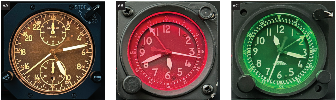
Figure 6. The three colors of cockpit lighting: A. Aerossonic model 88000-4102 in white; B. Waltham ABU-11/A in red; C. Thommen B18 in night vision green. AUTHOR'S PHOTOS.
