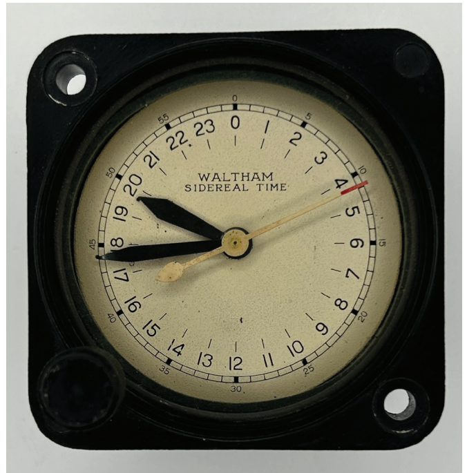
Figure 17. This rare Waltham A-11 was designed for astronomical expeditions and is regulated for sidereal time. AUTHOR'S PHOTO.
