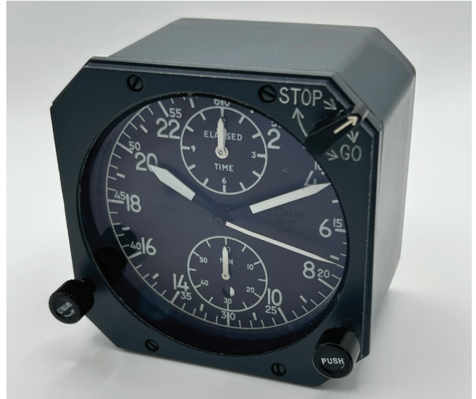
Figure 2. The Aerosonic clock used in Boeing 707, 727, and 737 aircraft during the pre-digital era. AUTHOR'S PHOTO.
