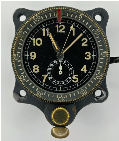
Figure 5. An early Jungheims Bo-UK1 version 2 clock. European military planes used several iterations of this clock design. Sinn and others improved on the design while maintaining interchangeability. AUTHOR'S PHOTO.
