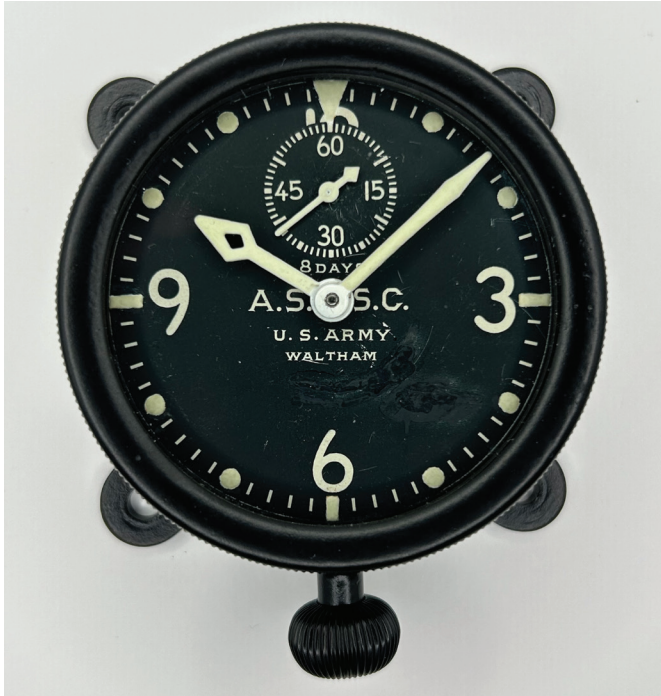
Figure 7. A Waltham XA made for the US Army Aviation Section Signal Corps. AUTHOR'S PHOTO.
