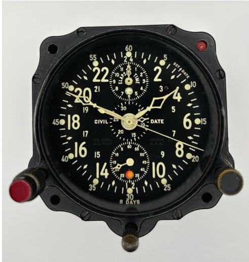
Figure 3. The Jaeger Chronoflite was produced during the 1930s through the 1950s and was the clock of choice for many aircraft flown by the Army Air Corps, Navy, and Royal Air Force. AUTHOR'S PHOTO.
