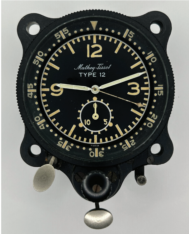
Figure 12. Like Breguet, Mathey-Tissot built a case and dial but relied on Valjoux for its aircraft clock movements. The parts are still available today. AUTHOR'S PHOTO.
