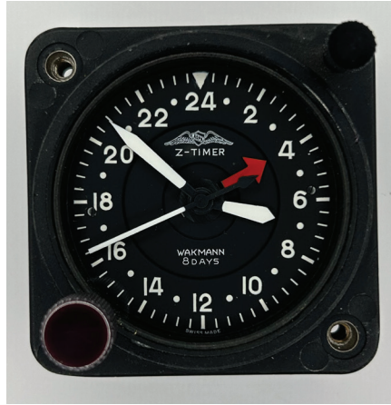
Figure 10. The Z-Timer ensured that a pilot would never lose track of Coordinated Universal Time, formerly known as Greenwich Mean Time. AUTHOR'S PHOTO.
