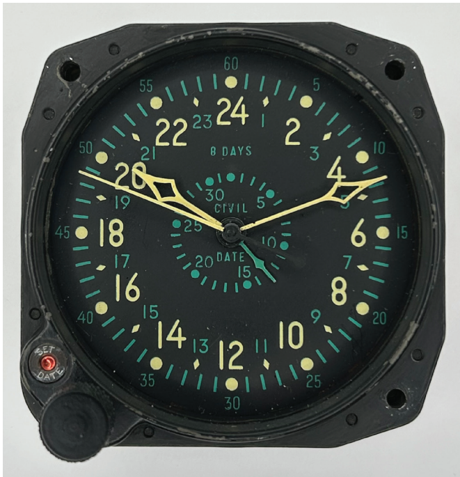
Figure 16. The CDIA clock was used in a wide variety of World War II aircraft. It was replaced by the Elgin-Hamilton 37500, which was designed with the same mounting configuration. AUTHOR'S PHOTO.
