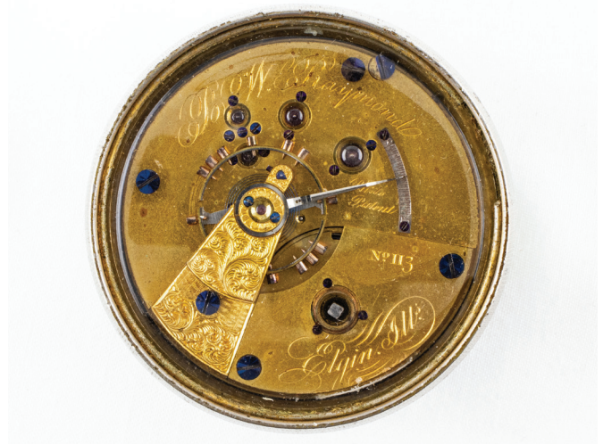
Figure 7. Elgin's first run of movements was the B. W. Raymond model, grade 69, 18-size, key wind and set, 15 jewels. Serial numbers began with 101. The first few dozen movements were given to some of the initial investors and a few others associated with the company's start-up. This watch, serial No. 113, was presented to John C. Adams, who was later involved in the start-up of at least four other watch companies. PHOTOS COURTESY OF THE ELGIN HISTORY MUSEUM.
