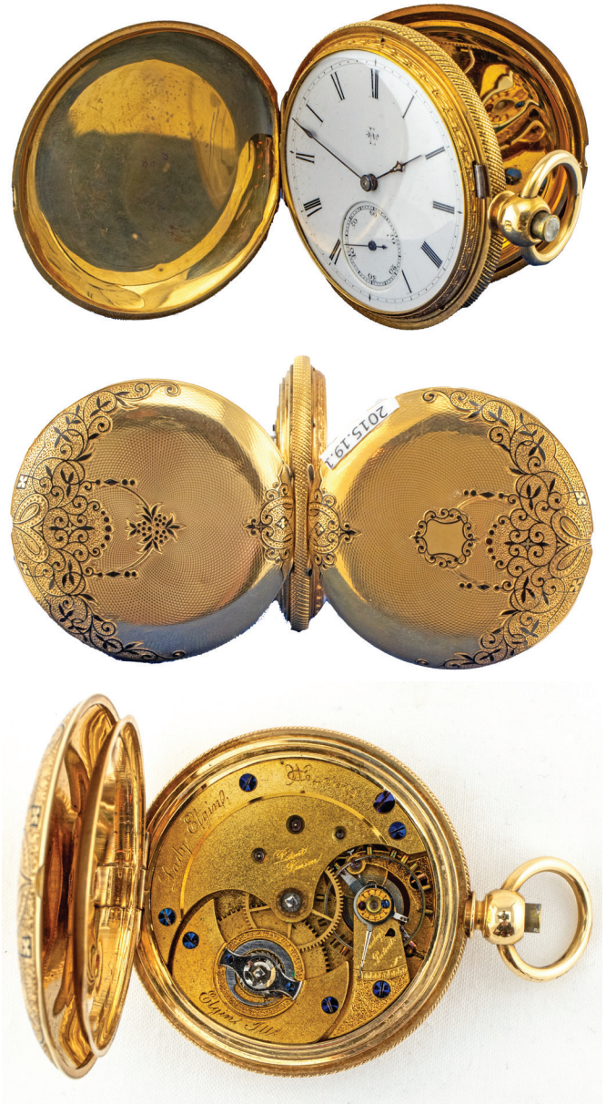
Figure 1. Elgin's first watch for the ladies' market was manufactured in 1869. This is the third movement, serial No. 40,003 (10-size, key wind and set, 11 jewels, gilded plates). The watch was given to Orlando Davidson, a board member of the company and prominent Elgin, IL, businessman. He served the community in a number of ways through his civic leadership. The watch was for his wife, Caroline, who was the daughter of the city's founders, James T. and Laura Gifford. PHOTOS COURTESY OF THE ELGIN HISTORY MUSEUM.
