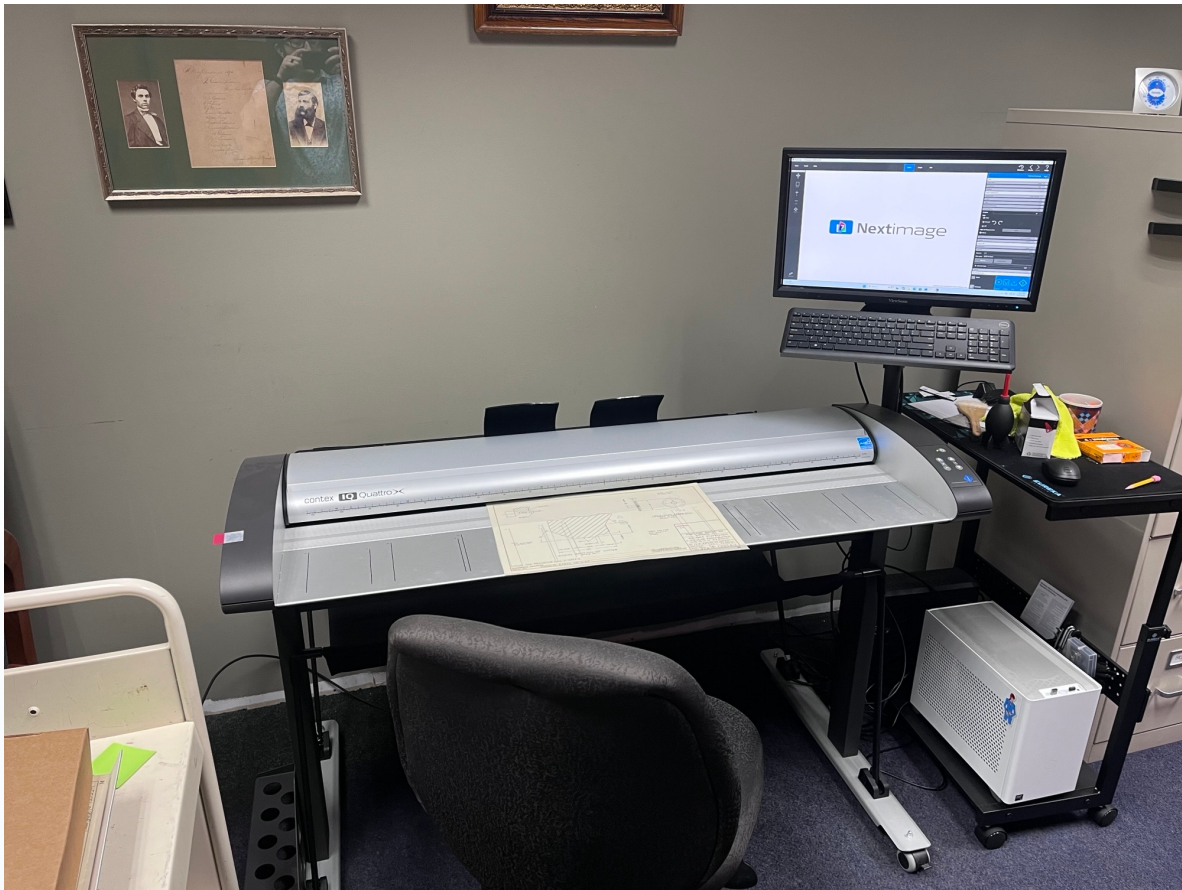
A Context IQ Quattro X 4450 44 scanner used for scanning large documents.
