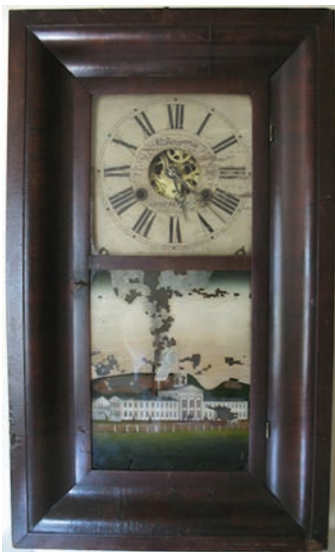
Figure 5. The simple mahogany veneered S-shaped (ogee) case with a 1-day or larger 8-day weight-driven brass movement was made by the thousands from the late 1830s into the 1850s by Jerome firms and many others. This example has an original lower-door glass with a view of Jerome's New Haven factory where it was made. PHOTO COURTESY OF MIKE BAILEY, JEROMECLOCKCOLLECTOR.COM.
